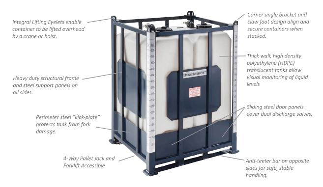
**DOT UN31HA1W Certified** for shipment of compatible multiple materials, which may not generate explosive, flammable, or poisonous gases if mixed. For additional details, reference CA2015030032 in UN/DOT information available at snydemet.com
