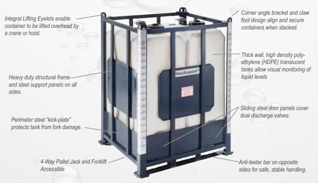
**DOT UN31HA1W Certified** for shipment of compatible multiple materials, which may not generate explosive, flammable, or poisonous gases if mixed.
